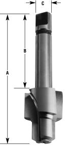
These tools have three flutes which form the standard internal O-Ring Boss for straight thread tube fittings. Standard in high-speed steel. Carbide tipped available on special order. Four flute cutters available on special order.
